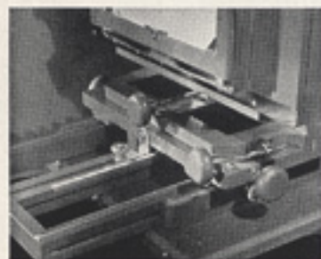
Special construction of camera and stand to permit all adjustments from focusing position.
